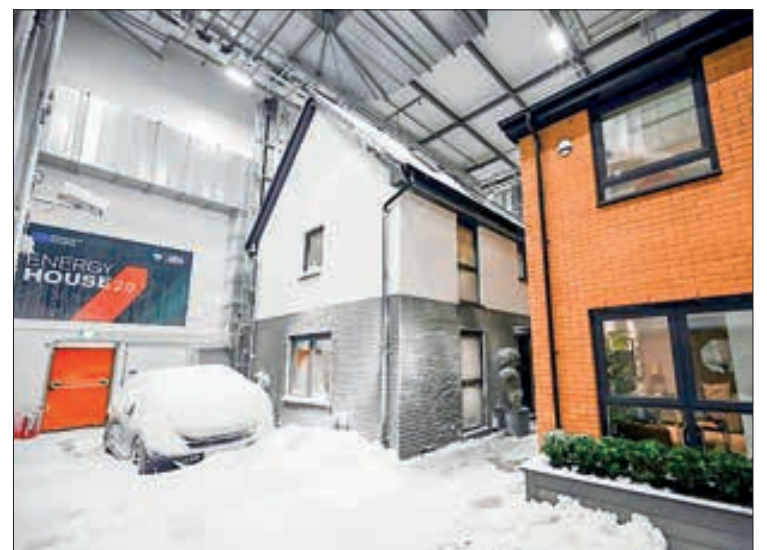
Simulated snow covers a car and the walls of one of two houses built in a lab to develop future heating solutions that will use less energy and help meet climate goals. PHOTO: AFP
